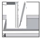
To cut, align an L square squarely to the board at the mark where you would like to cut. Run a utility knife along the edge of the L square to "score" the plank where you marked it. Then simply bend to "snap" along the score line. Run knife along fold line to separate into 2 pieces.
