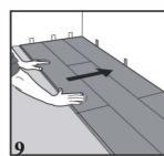
Adjust the distance to the walls when three rows are completed. Using spacers, place the flooring 1/4" from the walls. Keep the spacers in the entire installation and remove when complete.
