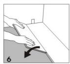
Place the plank at an angle against the plank in the first row, press forward and fold down at the same time. Leave the plank in a somewhat up angled position where the planks start to lock. To make this easier, a wedge with the suitable width can be placed under the plank near the short side.
