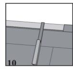
If the wall is uneven, the planks must be adapted to its contours. Mark the planks with the contour of the wall. Do not forget to leave a 1/4" space to the wall. This procedure can also be used for the first row if necessary.
