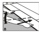
Lift plank together with the previous laid in the same row up a little over an inch and push it against the row in front. Put it down when the planks are tightly together. Continue this for three rows.
