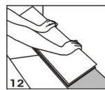
If necessary, re-lay the first row from left to right. Press the first board against the edge of the planks that are already in position.
