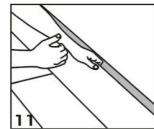
To remove the first row, lift the plank a few centimeters and tap along the joint. Cut the planks as required.
