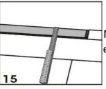
Measure and cut the last row to size. Allow for 1/4" expansion in your measurement.
